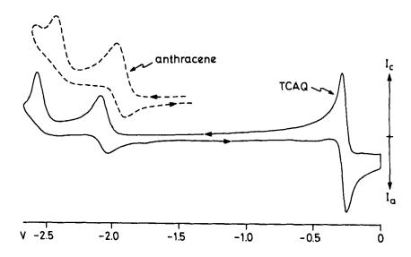
FIGURE 1 Cyclic voltammograms of TCAQ and anthracene. Solvent, acetonitrile; supporting electrolyte, Et<sub>4</sub>N<sup>+</sup>BF<sub>4</sub><sup>-</sup>; reference electrode, Ag/AgCl/KCl 3M: sweep, 200 mV/s.
